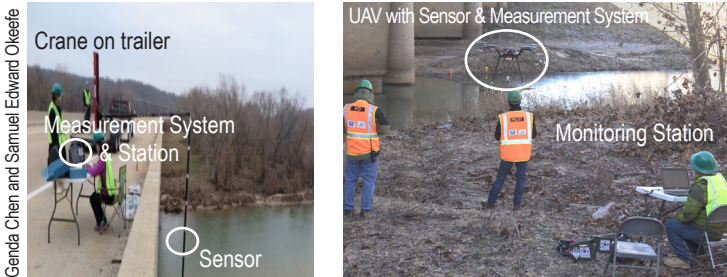
Figure 3: Magnetic field measurement with a sensor installed on a crane moving with the trailer or on a UAV.
